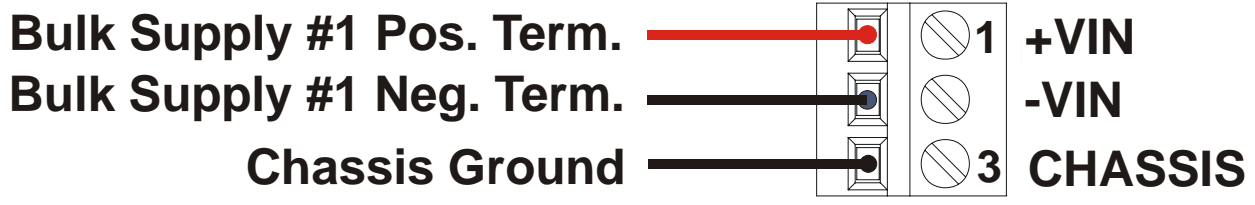
Figure C-2 - SCM Component Identification and TB1 Wiring Diagram
